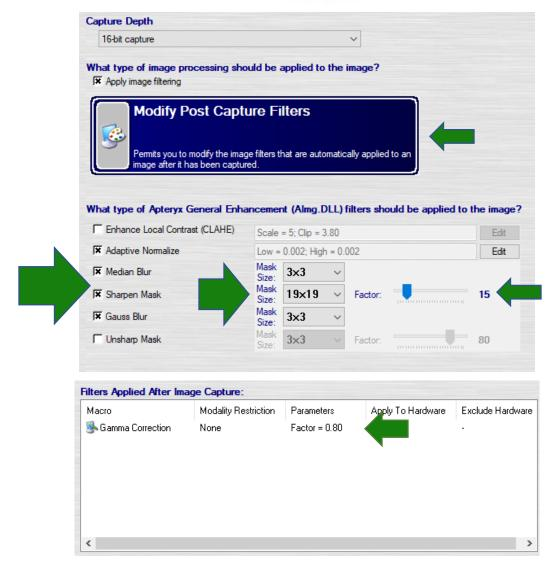
Double click on the Gamma Correction to adjust the Factor. If there are any other items in the Filters box, right click on each one and use "Delete Selected Filter" to remove it so that only Gamma Correction remains.
